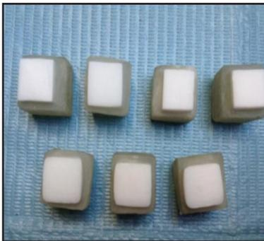
Fig. (5) Zirconia specimens embedded in acrylic blocks
