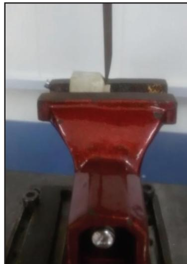
Fig. (13) Shear sample mounted on the universal testing machine for shear bond test using chisel edge blade
