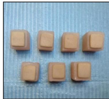
Fig. (6) Porcelain specimens for metal veneering embedded in acrylic blocks
