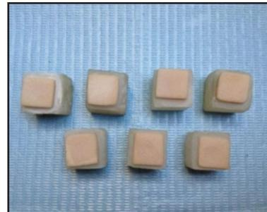
Fig. (7) Porcelain specimens for zirconia veneering embedded in acrylic blocks
