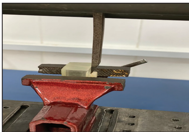
Fig. (1) A photomicrograph showing Sample mounted on the universal testing machine for shear bond test using chisel edge blade.
