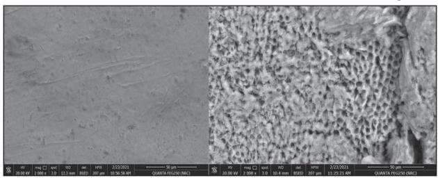
Fig. (2a): Scanning electron micrograph of sound untreated enamel preserved in artificial saliva showing smooth, regular enamel surface with barely evident rod and interterrod (2000xmag) vs Fig. (2b): Scanning electron micrograph of demineralized enamel surface show the rod with honeycombed pattern and interrod (mag. X 2000).
