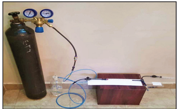
Fig. (1) A photograph showing assembled fluid filtration apparatus
